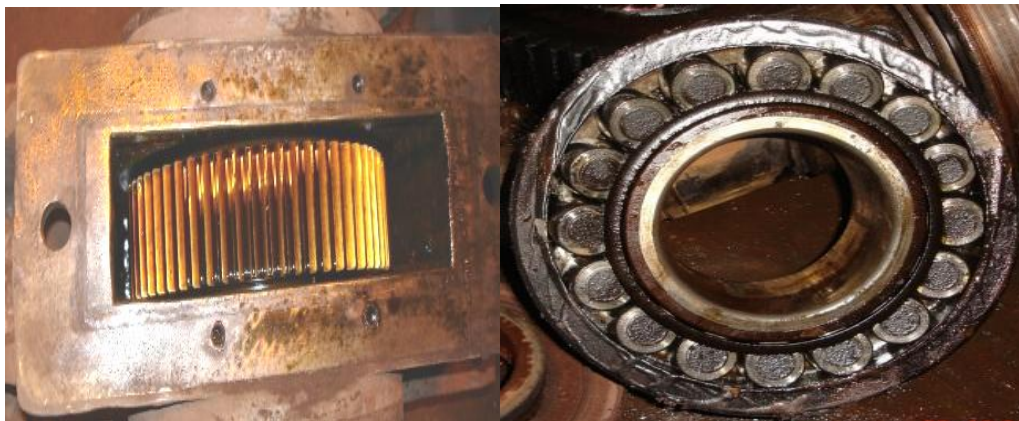
Photographs of burnt oil inside exciter gearbox and seized bearing
