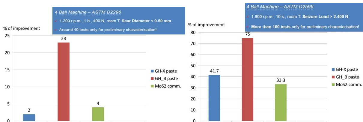
Fig. 19. Comparative testing of greases with 4-Ball machine. Left – according to ASTM D2296; Right – according to ASTM D2596
