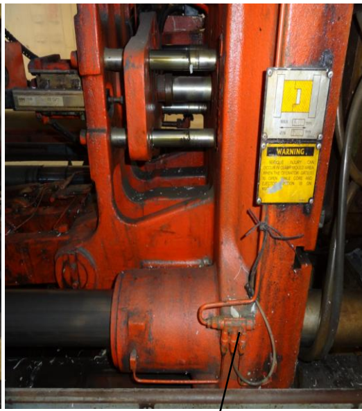
Distributor having very small orifice through which grease is pumped into the tie-bar
