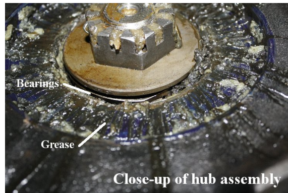
Figure 8. Excessive spillage of grease leading to lubrication starvation.
