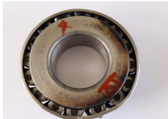
Figure 9. Oxidation due to overheating.
