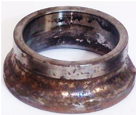
Figure 11. Pitting and corrosion due to mud ingress.
