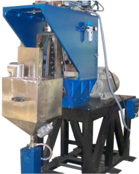
Figure 6. A hub bearing tester with dust attachment.
