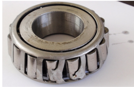
Figure 12. Entrapment of failed cage.
