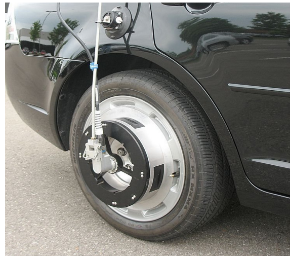
Figure 5. A passenger car fitted with a wheel force dynamometer.
