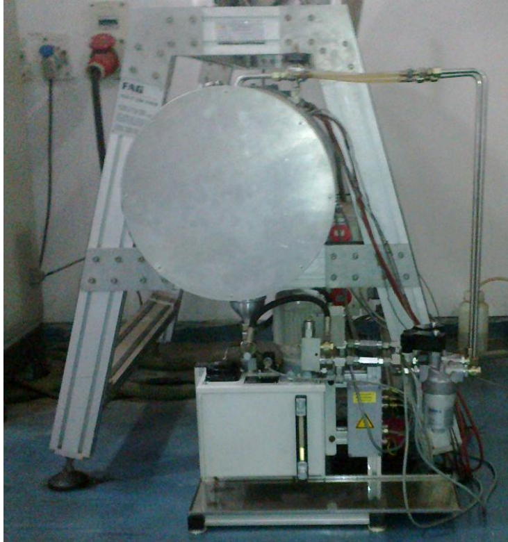
Figure 2: FE8 Test rig connected to an oil recirculation system
