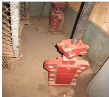
41mm Guide rope clamped in headframe
