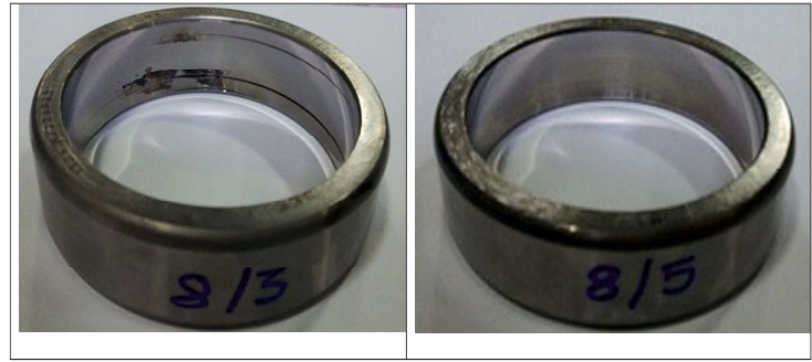
Fig 5: An example of rust rating during Emcor test
