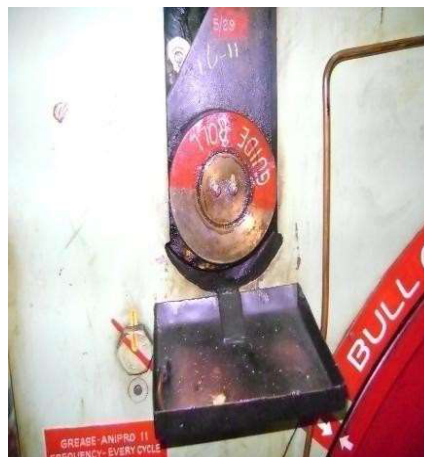
Fig-4: Side arm bearing: Old grease Fig-5: Side arm bearing: Newly developed grease
