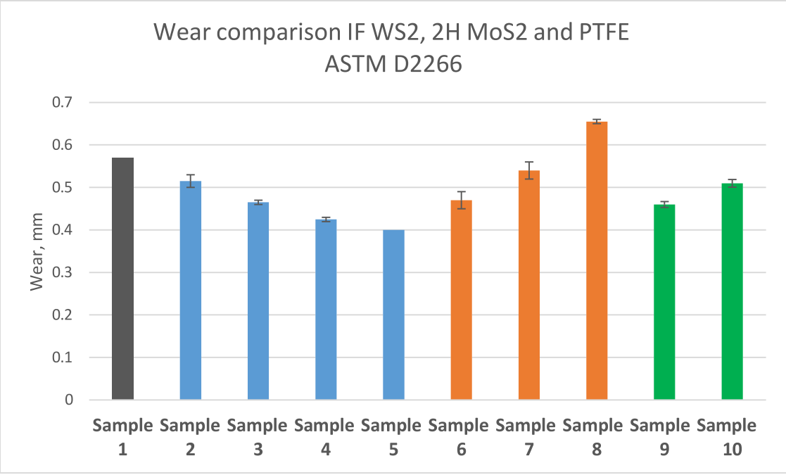
Figure 5. Wear scar comparison of tested samples
