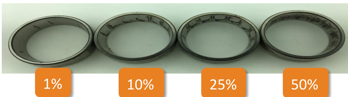
Figure 3 - Modified rust rating used in this study - percent surface coverage of corrosion
