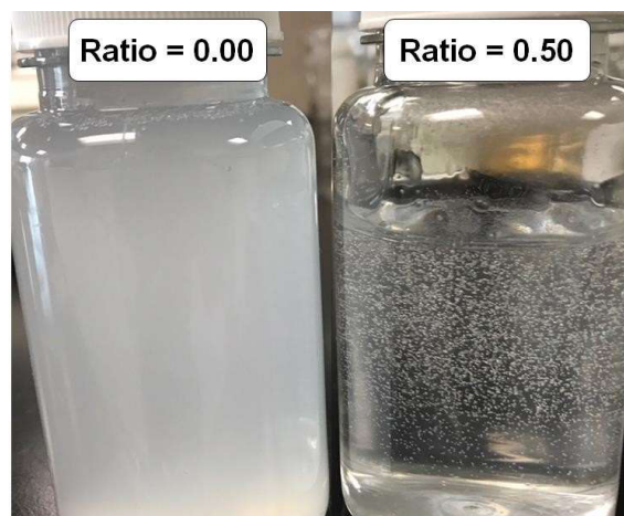
Figure 13: Haze in ISO 15 preparation of polyether polymer (PE3) with clarifier salt at varying mass ratios from 0 to 2.5. An optimal ratio is achieved at ratio = 0.5 (1 part clarifier to 2 parts polymer in water). The use of salt to reinforce solvent cage structure around the polyether polymer enables clear and concentrated PE water-based thickener with high VI.
