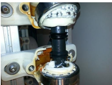
Figure-1: Grease color was changed during EMCOR test with distilled water
