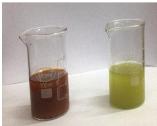
c) Color of the Ester Sample E after RBOT test with both types of Antioxidant
