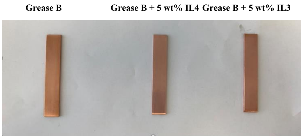
Figure 6. Copper strips after exposure to neat grease B and formulations with 5 wt% of IL3 and IL4 respectively.
