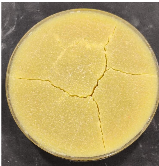
Fig 4: Caking effect of grease after 12 hours at 120°C (Complexing calcium grease with different acids)
